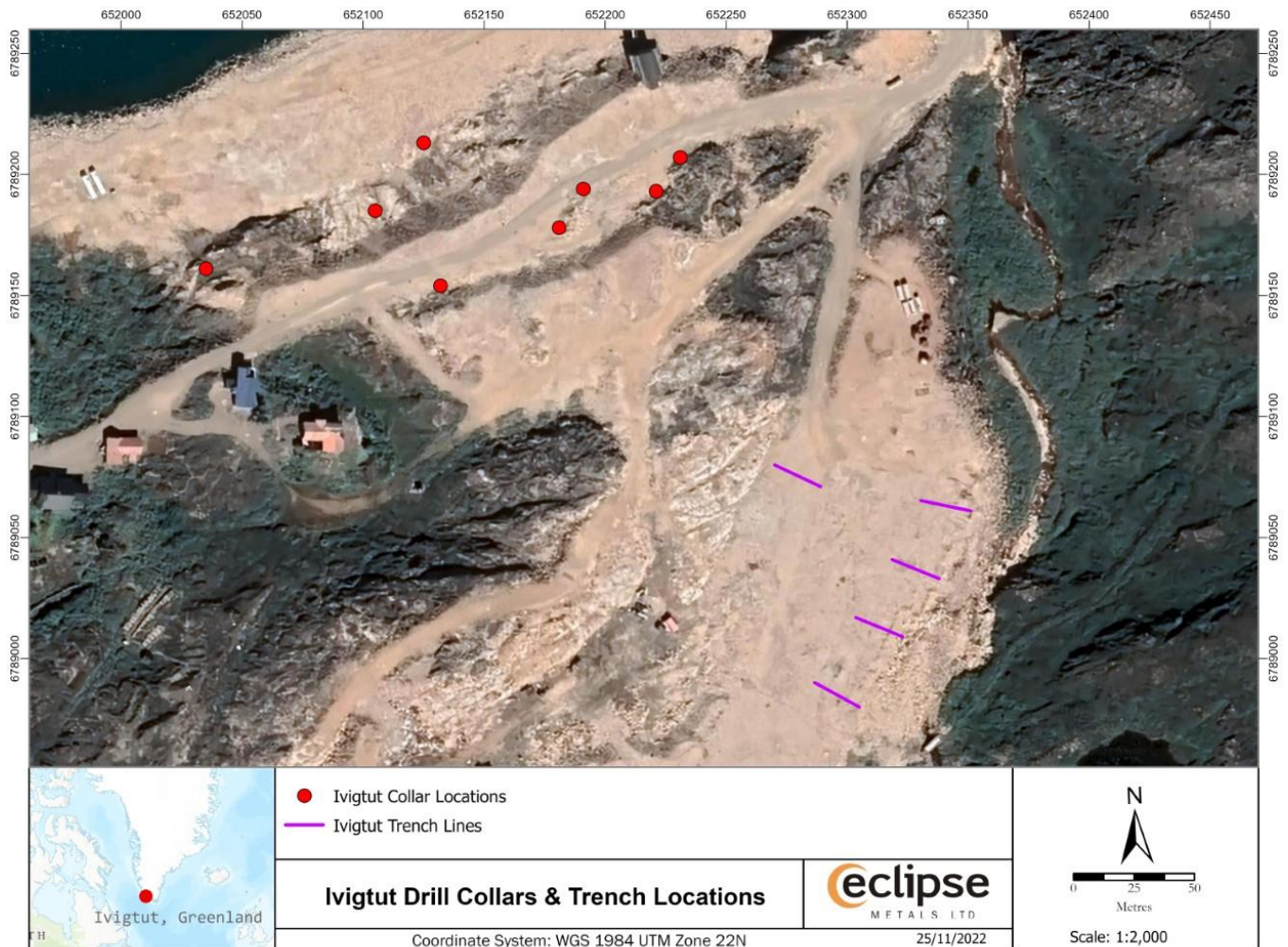
Figure 6: Ivigtut target area. Drill collars are marked with red dots. Bulk sample trenches are marked with purple lines. Assays are expected to be available toward the end of Q1 2023
