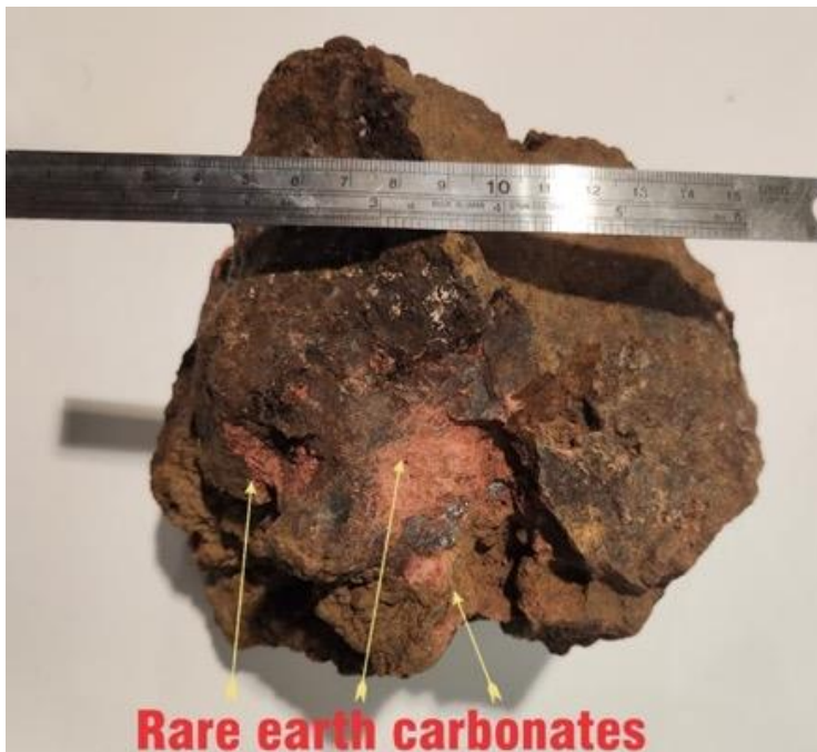
Figure 1: Grønnedal surface sample shows pink/orange REE mineral. Visually estimated to comprise of ~25% pink-orange material and 75% iron oxides and oxidised carbonatite.
