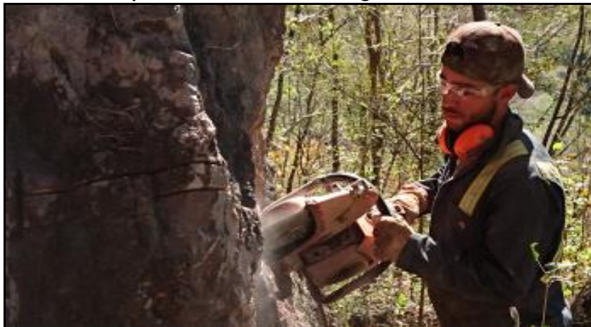
Photo 1. Example of Diamond Saw Cutting for Continuous Channel Sampling
