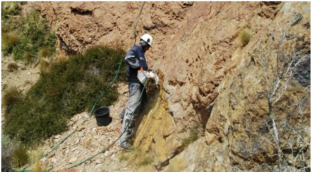
Photo 1. Diamond Saw Cutting for Continuous Rock Channel Sampling at Los Domos
