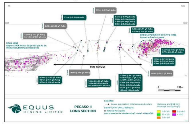
Figure 12 - Pegaso II Long Section: showing drill hole vein pierce points based on Equus and historical drill results.
