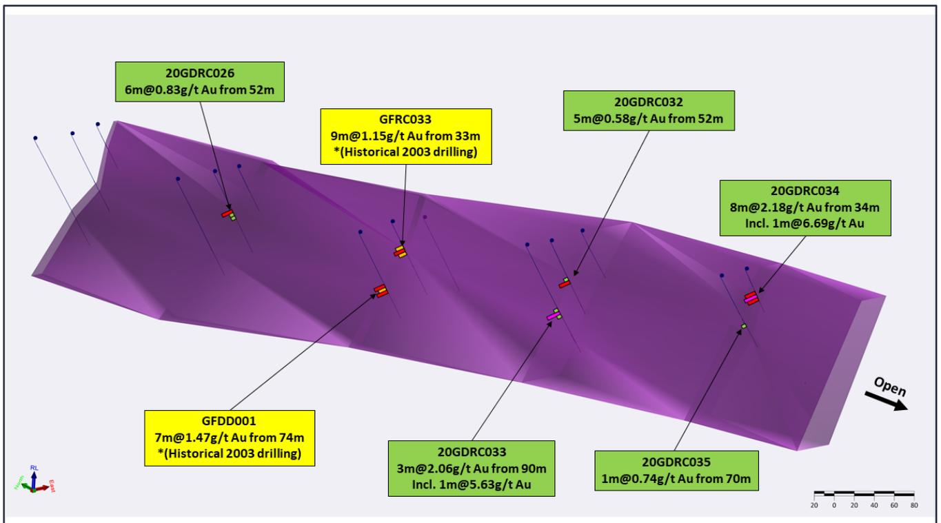
Figure 3 – Oblique long section looking northeast showing the modelled Gards Porphyry (purple wireframe) and significant intercepts from December 2020 drilling (green labels) and historic 2003 Placer Dome drilling (yellow). Mineralisation is open to the southeast.
