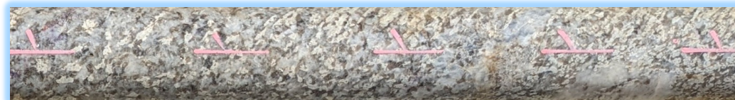
Example of drill core taken from the upper zone of the Cade Deposit illustrating the relatively homogenous mineralised pegmatite and some weathering on fractured sections (Hole ID PDD598).
