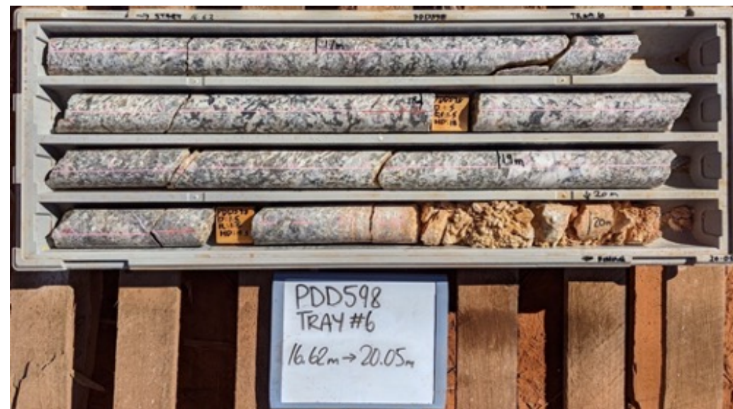
Example of drill core taken from the upper zone of the Cade Deposit illustrating the relatively homogenous mineralised pegmatite and some weathering on fractured sections (Hole ID PDD598).
