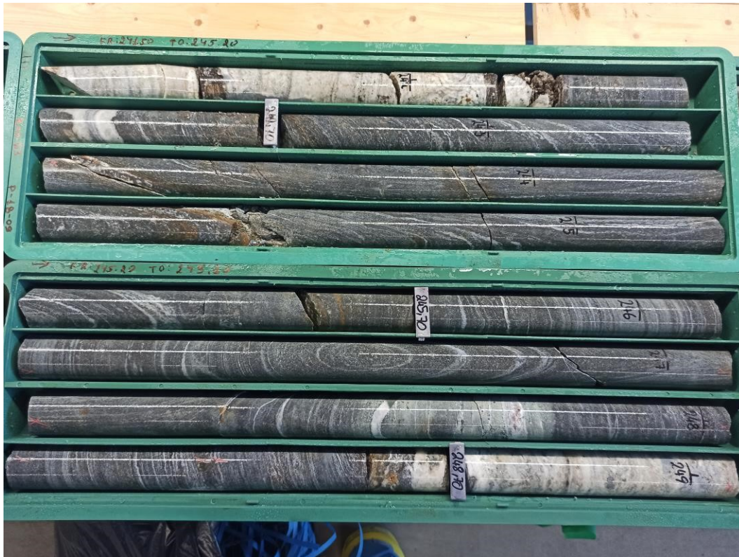
Picture 3: 2 AHP veins, vein @ 248.7 m contains big spodumene crystals (continue next picture)
