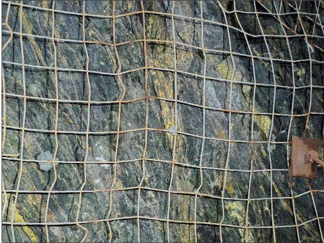
Figure 11: Stringer-style Footwall mineralisation from the 735 Level in the Ming Mine (photograph taken in September 2024). The mineralisation consists of individual mm to cm scale chalcopyrite-pyrite veins hosted within highly chloritized rhyolite. This mineralisation is amenable to large-scale mining and often bulks out to grades exceeding 2% copper.
