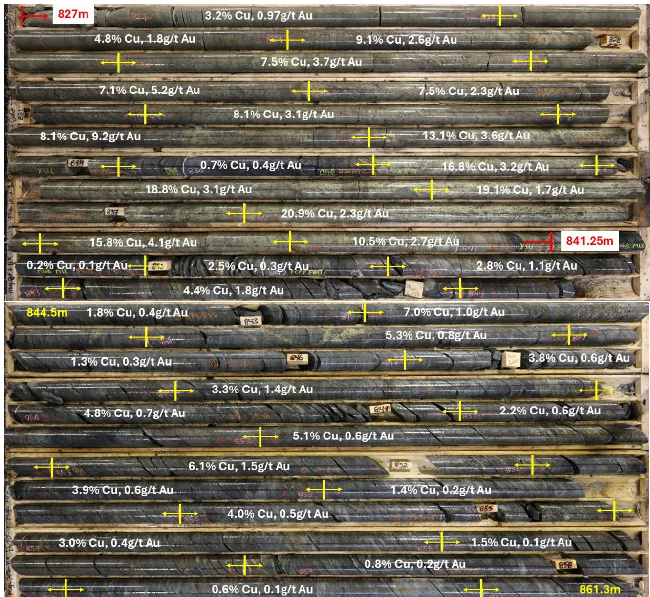
Figure 2: Core photographs for drillhole MUG25-202, showing the upper VMS (827m-841.25m) that grades 14.3m @ 13.7% CuEq and the adjacent broad FWZ stringer-style mineralisation. This is part of the broader step-out intersection of 49.0m @ 6.1% CuEq.
