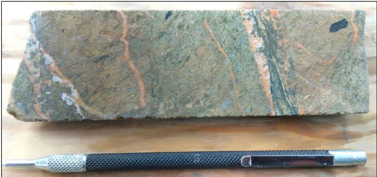
Figure 5: Quartz-carbonate-pyrite-arsenopyrite-cobaltite-scheelite-chalcocopyrite veins in altered crystal-lithic tuff, 2019FTD006, 106.7m (106-107m: 1.0m @ 5.71/t Au, 0.23% Co, 0.88% WO 3 and 0.25% Cu).
