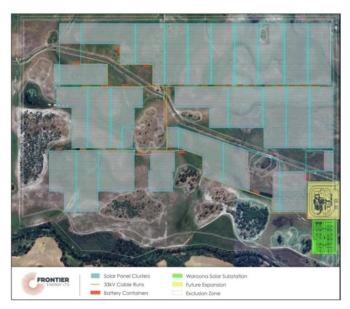
Figure 10: Waroona Solar Farm Stage One layout
