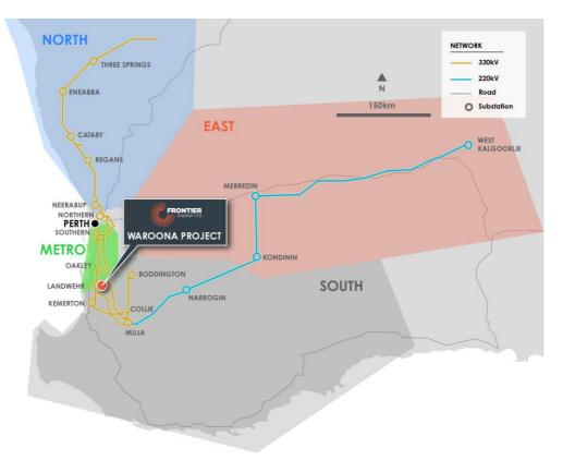
Figure 5: SWIS 330kV and 220kV networks
