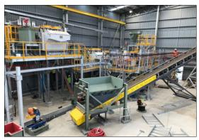
Figure 4 - View Inside Process Building looking east. With flotation area in the background and dryer feed conveyor in the foreground.
