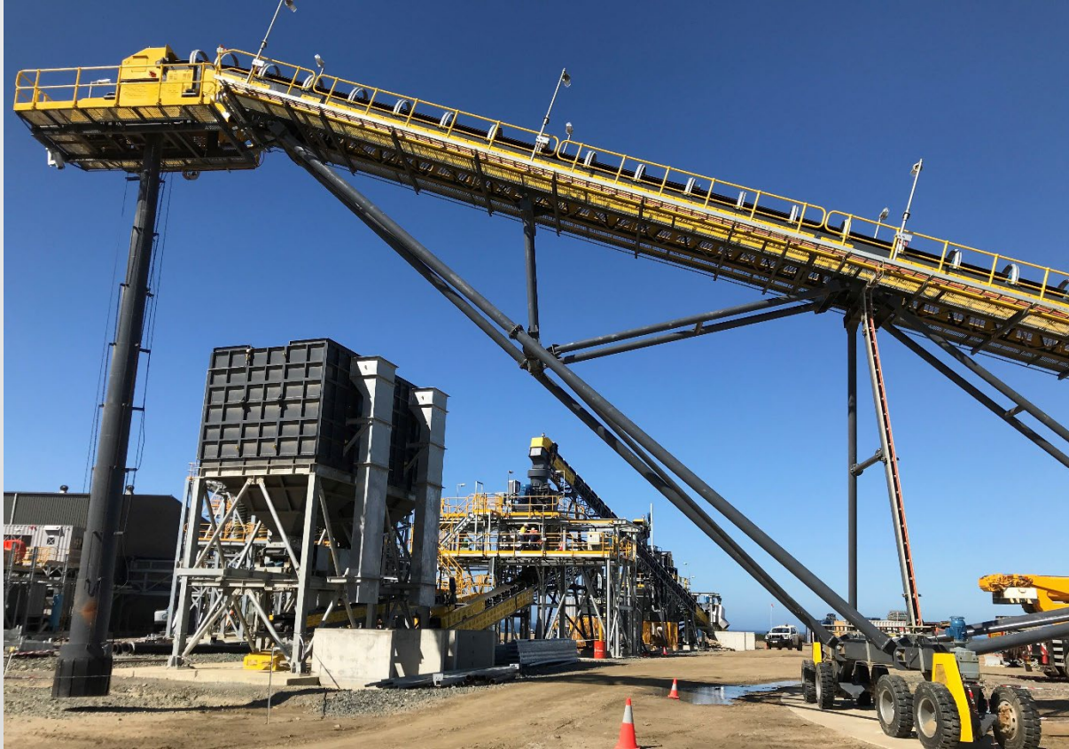
Fine ore stacker, fine ore bin and tertiary crushing and screening circuit
