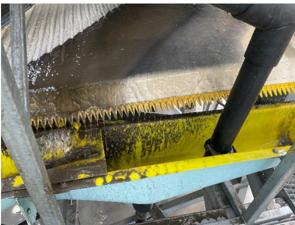
Figure 4 - Tungsten Separation on Shaking Tables
