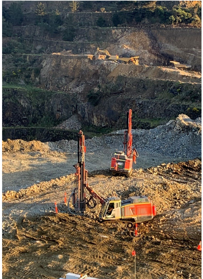
Figure 2 - East Pit Overburden Drilling
