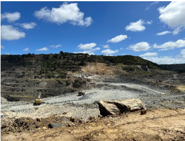
Figure 1 - Preparation of benches on the eastern side of the Dolphin Pit for mining of high-grade ore
