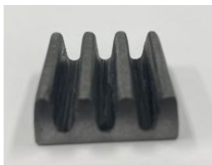
Figure 1 - VHD Technology Prototype Heat Sink
