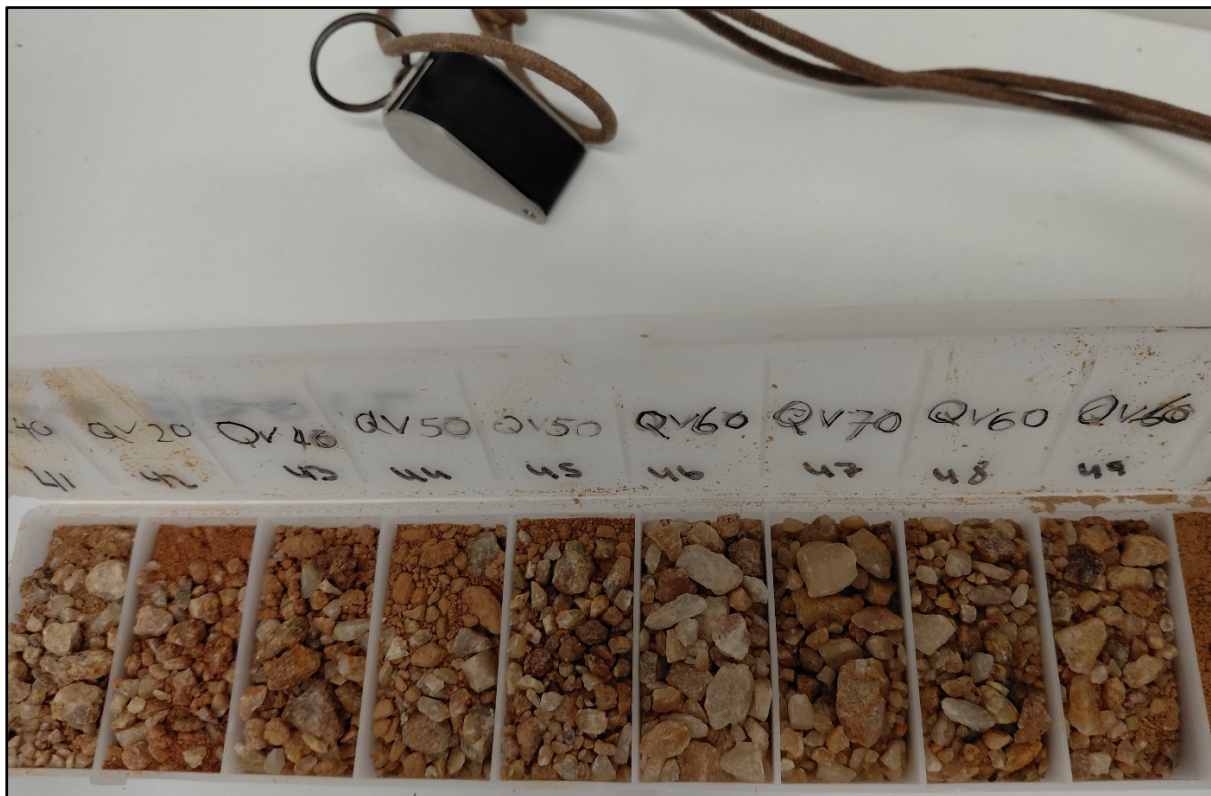
Figure 2. Drill hole chip tray of 26BB012 highlighting the quartz rich high-grade interval of 4m @ 4.36 g/t Au from 44m
