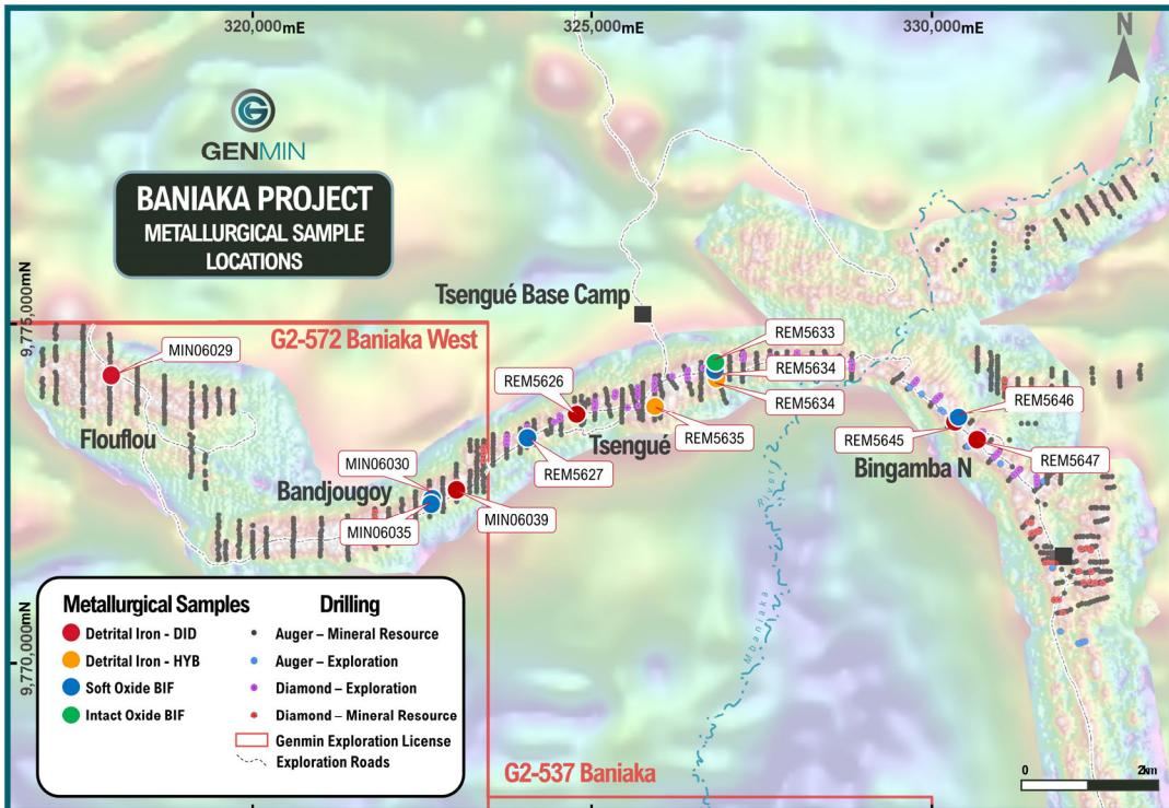
**Figure 3: Prospect scale location map showing Bulk Sample locations and drill traverses overlain on ground and airborne magnetic data**
