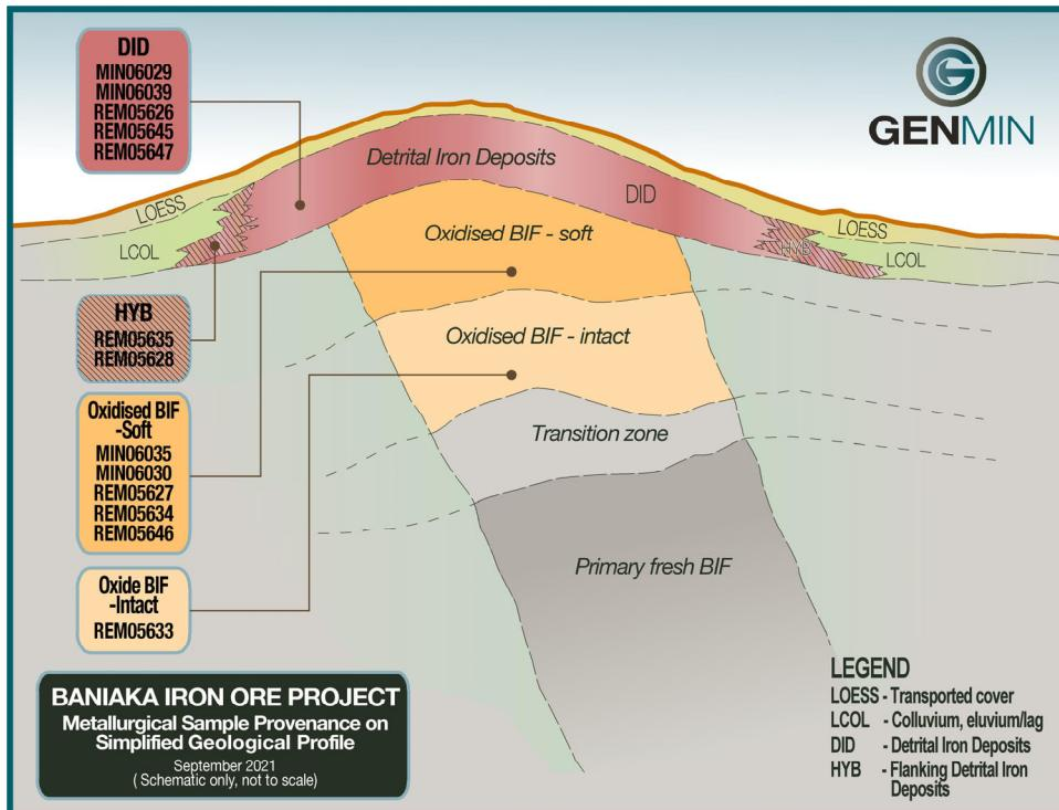
**Figure 4: Schematic cross section of Baniaka iron ore mineralisation, showing respective mineralisation zones for Bulk Samples selection**
