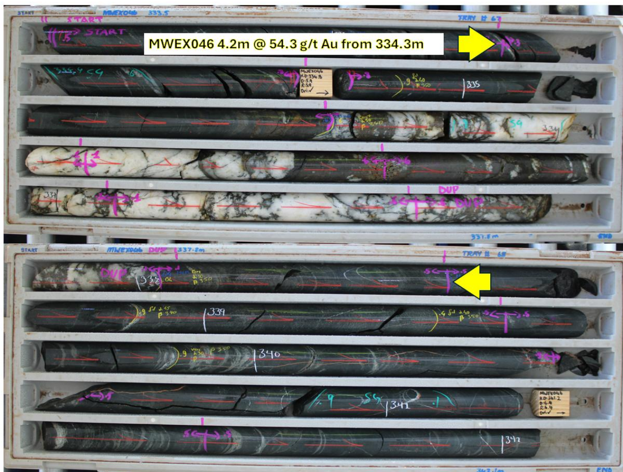
Figure 3. Example of gold lode at Mulwarrie in drill core, from MWEX046 334.3m to 338.5m; 4.2m @ 54.3 g/t Au
