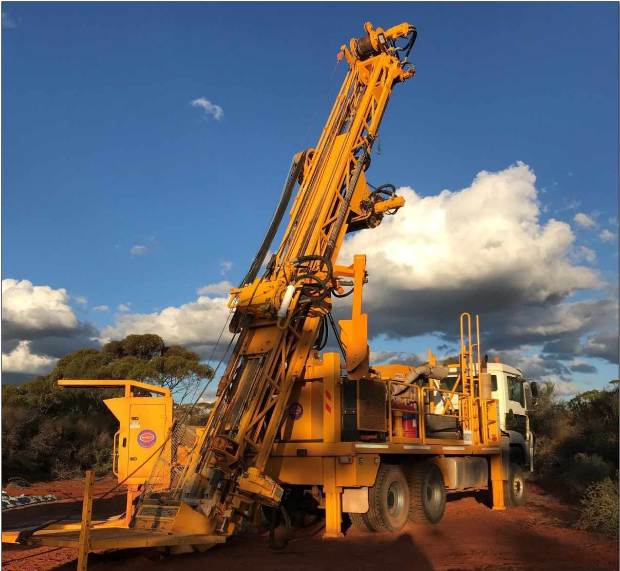
Figure 3 – Mt Magnet Drilling diamond rig at the Manna site
