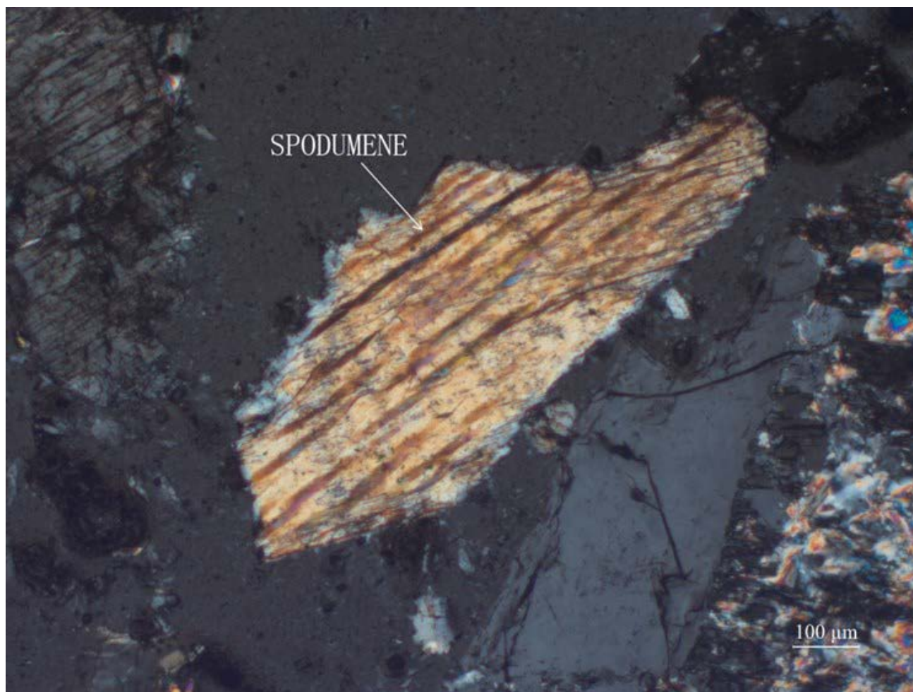
Figure 1. Electron microscope image of a Lithium bearing Spodumene monocrystal from the Marble Bar metallurgical test work.
