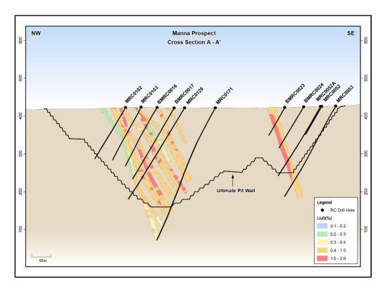
Figure 4: Manna cross section A - A' showing estimated Li₂O grades
