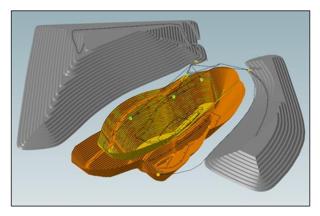
Figure 11: Haulage analysis shown for final pit stage
