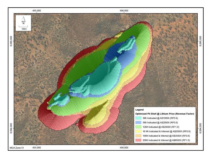
Figure 6: Optimised pit shells at different lithium prices
