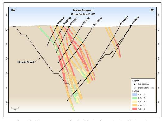
Figure 5: Manna cross section B - B' showing estimated Li₂O grades
