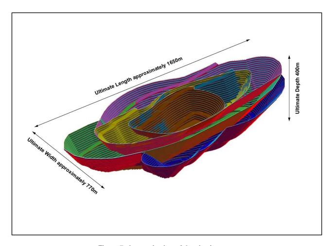
Figure 7: Isometric view of the six pit stages
