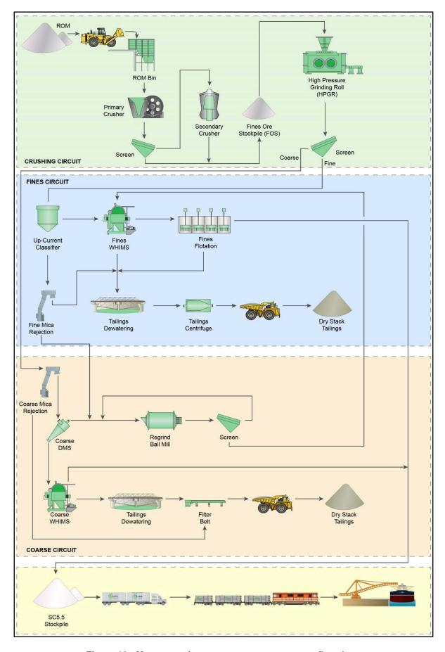
Figure 12: Manna spodumene concentrate process flowsheet
