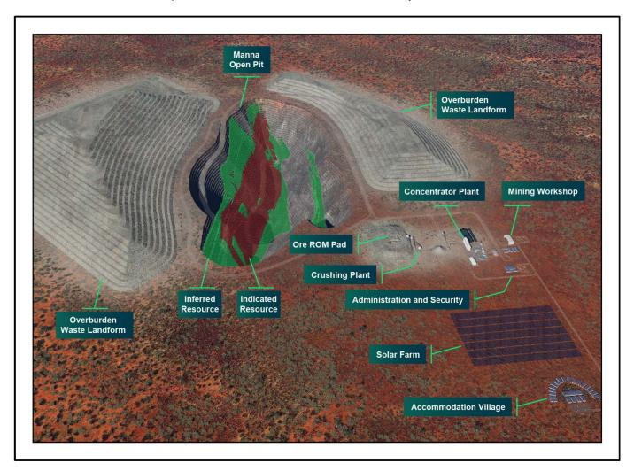
Figure 8: Final mine design with overburden waste landforms
