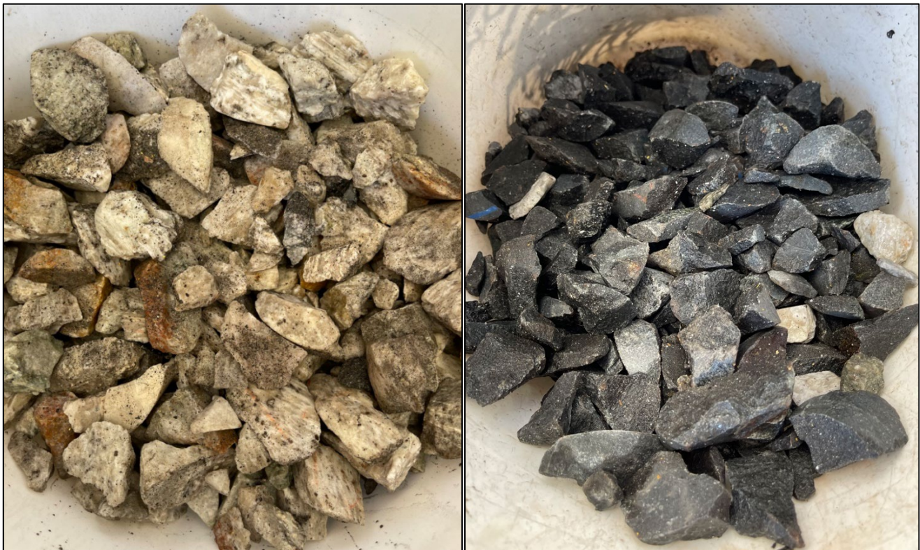
Figure 2. Ore sorter product streams, Accepts (Left) and Rejects (Right)
