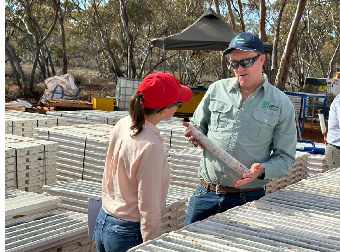
GL1 diamond core yard at the Manna Lithium Project site
