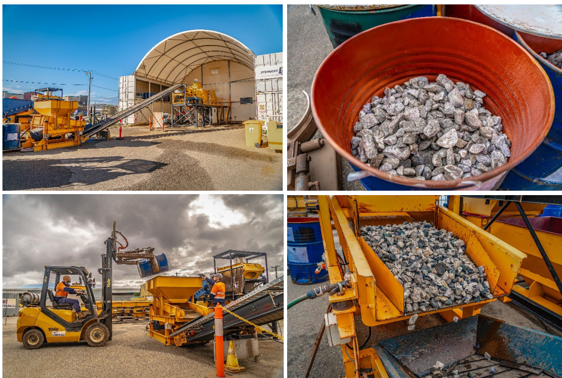
Figure 1. shows the high-grade ore being processed through the Steinert ore sorting facility.
