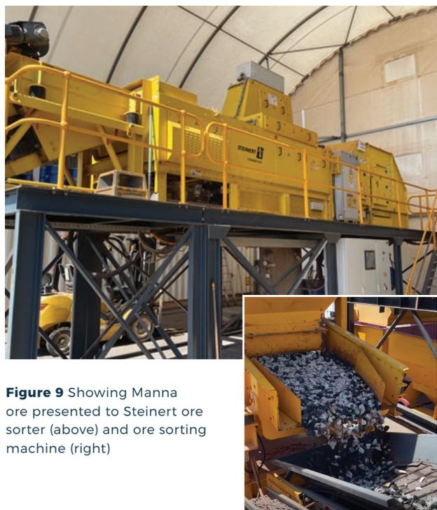
**Figure 9** Showing Manna ore presented to Steinert ore sorter (above) and ore sorting machine (right)
