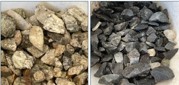
**Figure 10** Ore sorter product streams, Accepts (left) and Rejects (right)
