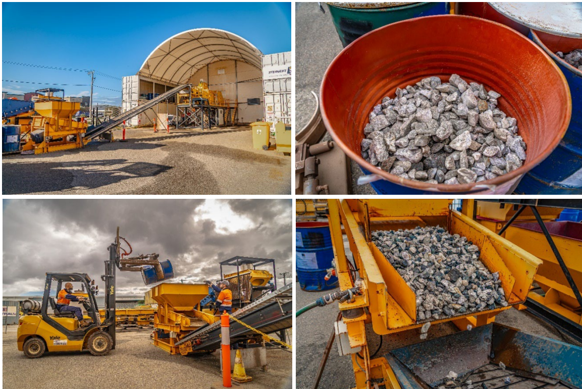
Figure 9. shows the high-grade ore being processed through the Steinert ore sorting facility.
