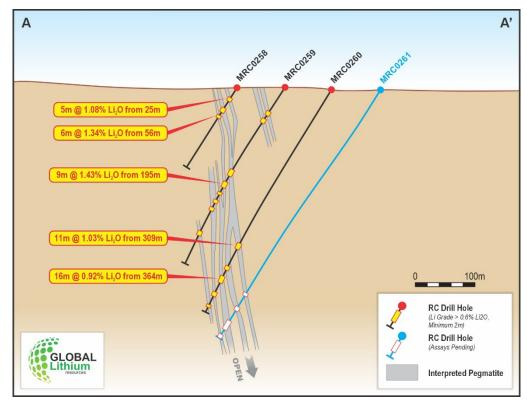
**Figure 2.** Cross section A-A' through the northern extension of the Manna lithium deposit with significant Li<sub>2</sub>O intercepts.
