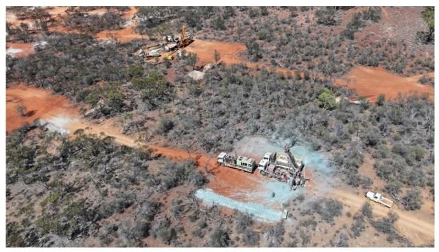
Figure 5. Infill drilling using multiple drill rigs at the Manna Lithium Project.
