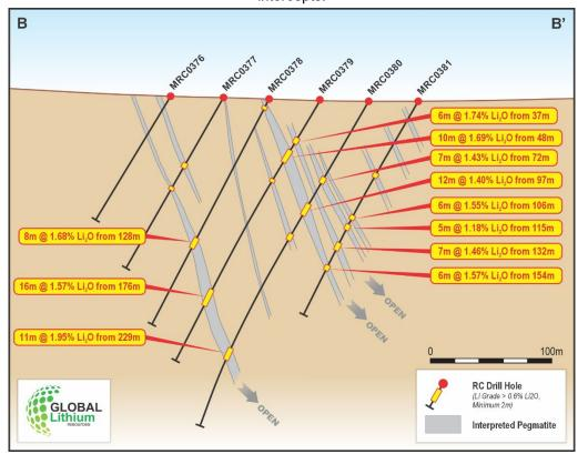
Figure 3. Cross section B-B' through the Manna lithium deposit with significant Li<sub>2</sub>O intercepts.
