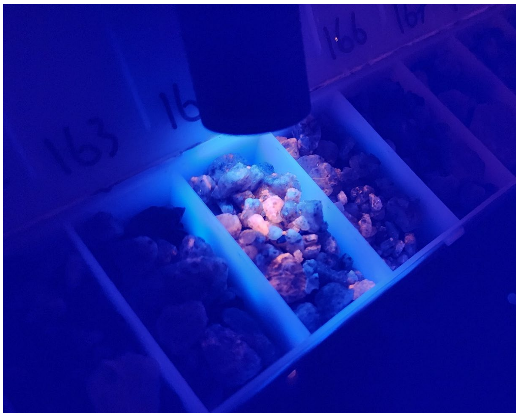
Figure 1: Spodumene fluorescence (orange colour) under UV light from 163-164m (0.99% Li 2 O) in hole MRC0451.
