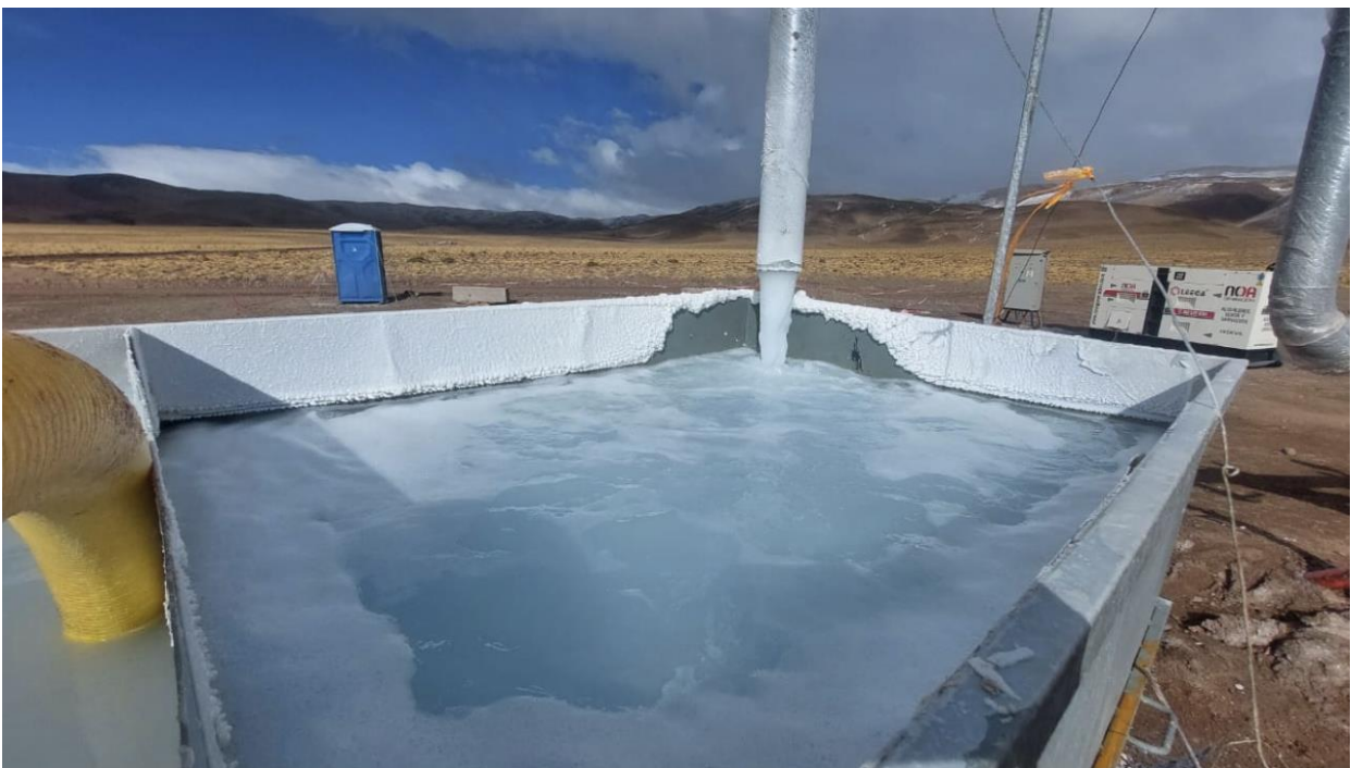
Figure 3 – Brine discharge at PPB-01-21 during long term pumping test.
