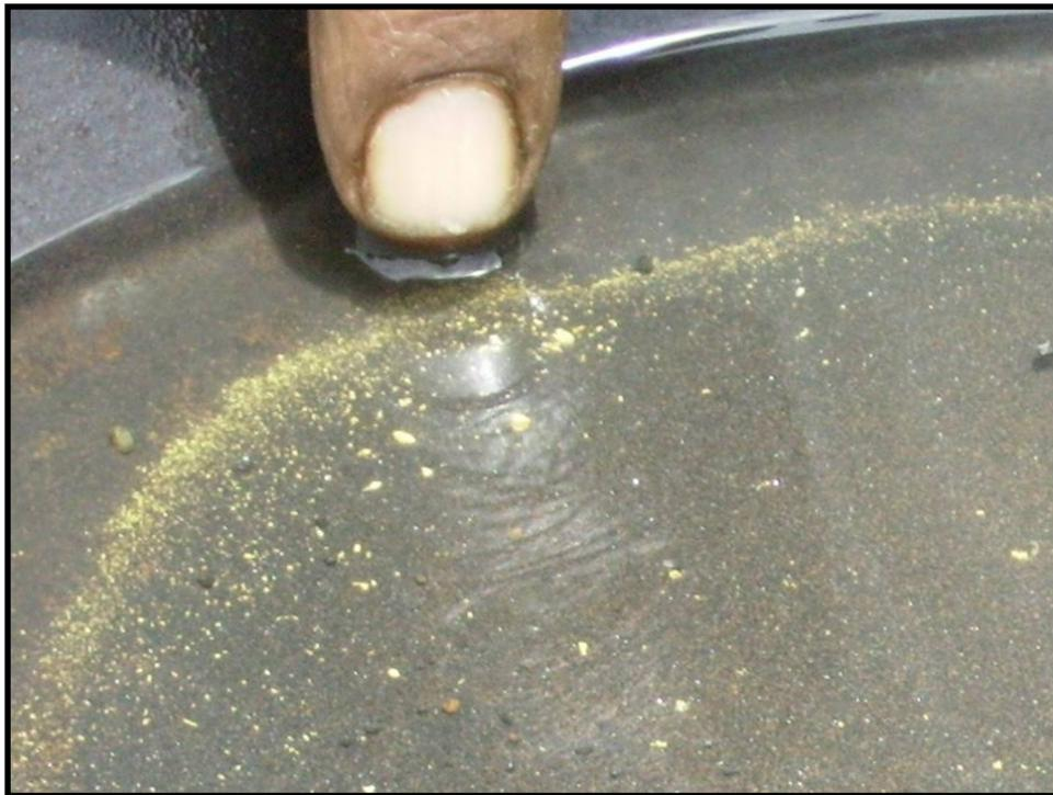
Figure 3. Gold in sample pan from crushed outcrop at Ista's Prospect.
