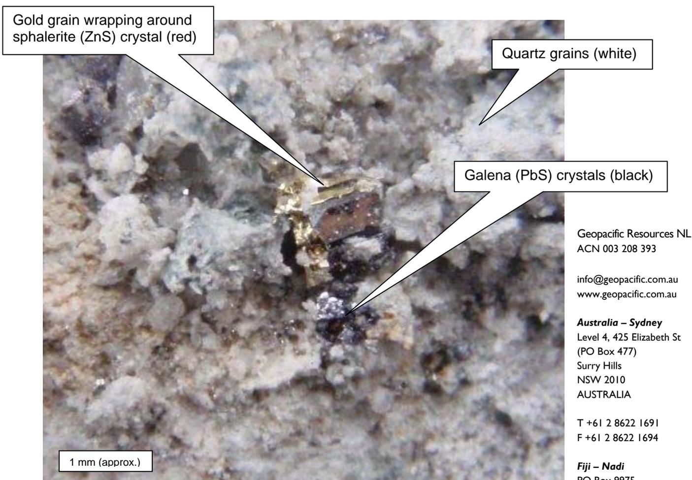
**Figure 1. Photograph of drill core near 43.5m in FAD045 showing platy gold grain partly enveloping a red sphalerite crystal (1 millimeter scale bar is approximate).**
