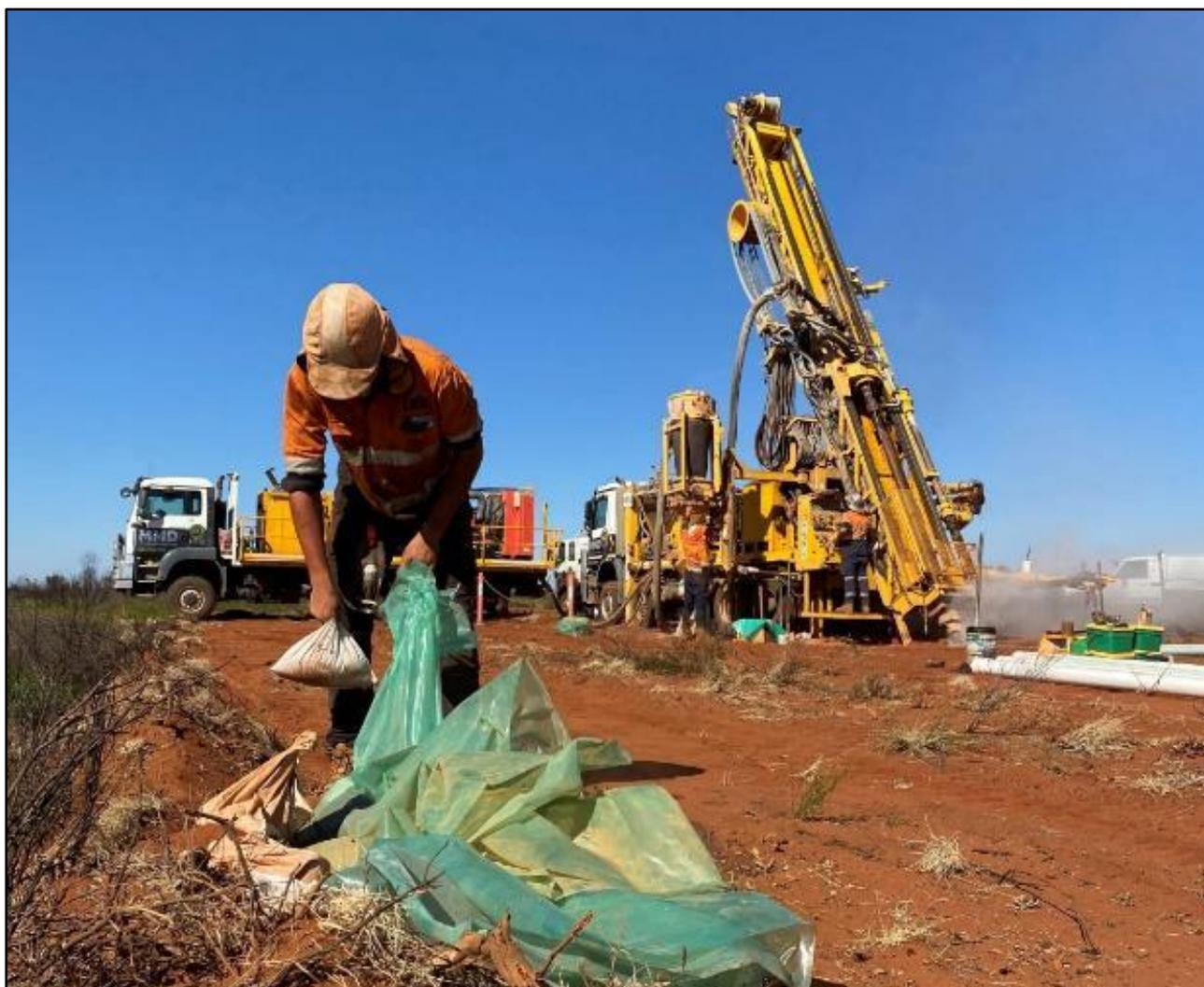
Figure 5: RC drilling at the Yule project's Nomad lithium prospect.
