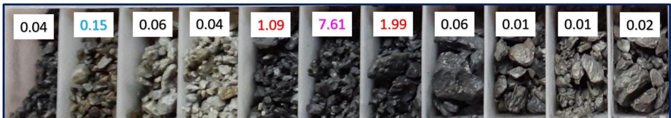
Figure 4: 20CFRC005 chip tray photo highlighting the high-grade interval at the lithological contact
