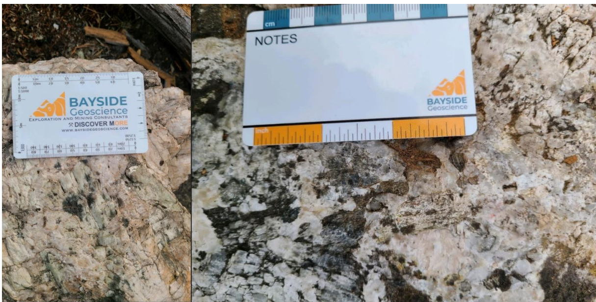
Figure 8: Tape Lake pegmatite exposure hosting coarse spodumene laths
