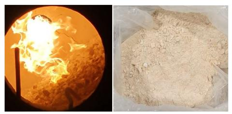
Figure 6: Rotary kiln start (LHS) and end (RHS) bulk calcination test Comp 2
