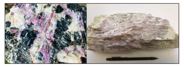
Figure 1 – Lithium bearing spodumene samples from Millie's Reward
