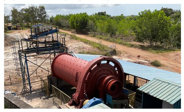
Figure 3 - Ball Mill #1 of Process Plant
