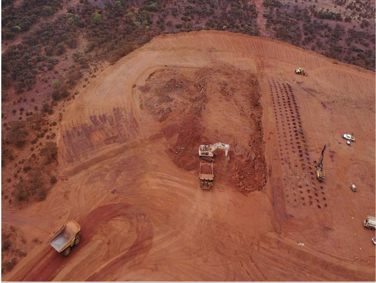
Figure 2: Drill blasting continues and material moved to the ROM pad.
