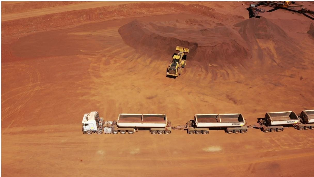
**Figure 1: Road Haulage Trucks being loaded with Stockpiled Iron Ore**
