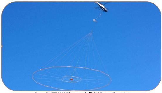
Figure 7: VTEM MAX<sup>™</sup> system in flight (Photo – Geotech)
