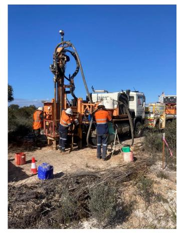
Figure 6: Drilling of hole AC198 Cowalinya project on 12/10/2022. Location: 6358205N 429402E. Total depth 46 metres.
