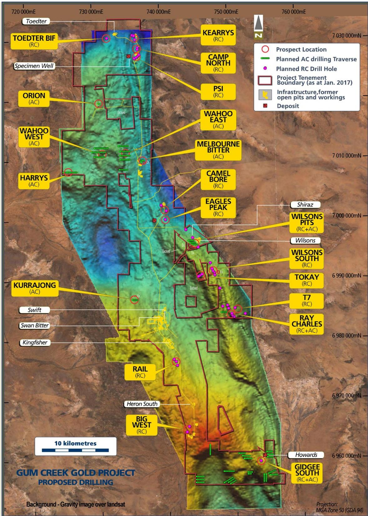
Figure 4: Colour gravity image showing prospect areas targets proposed for drilling in FY2018 (project tenure as at the date of the Prospectus)
