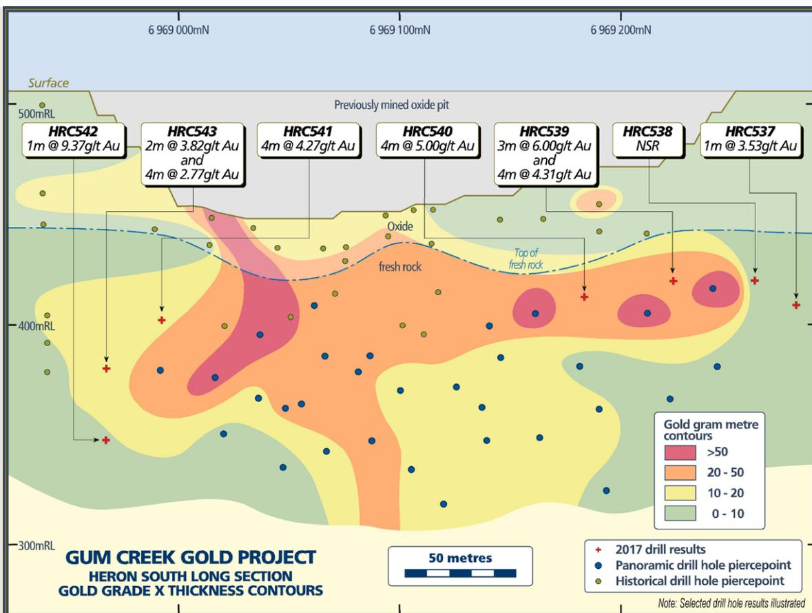
Figure 5: Infill RC Drill results at Heron South
