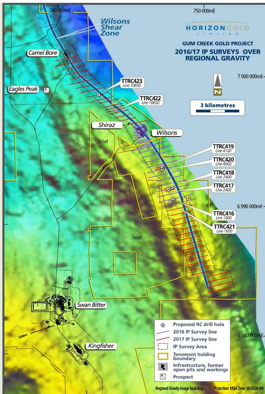
Figure 6: Gravity image showing Wilson's Shear IP survey lines and drilling completed in April 2017
