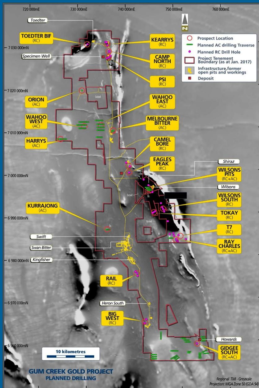
Figure 7: High resolution grey-scale Total Magnetic Intensity image of the Gum Creek Greenstone Belt, showing prospect areas proposed for drilling in FY2018 (project tenure as at the date of the Prospectus).
