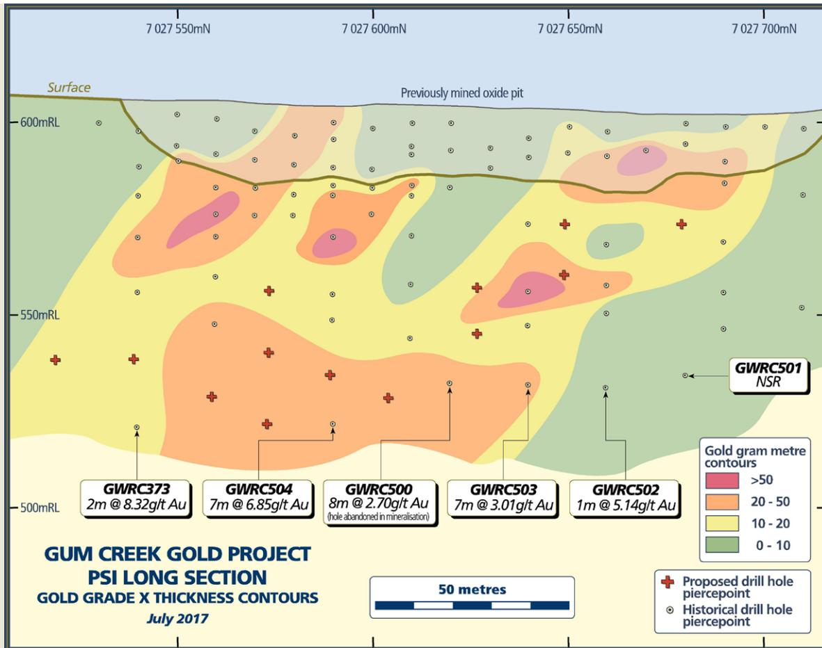
Figure 8: PSI Long Section showing thirteen planned RC holes to test depth extensions and infill
