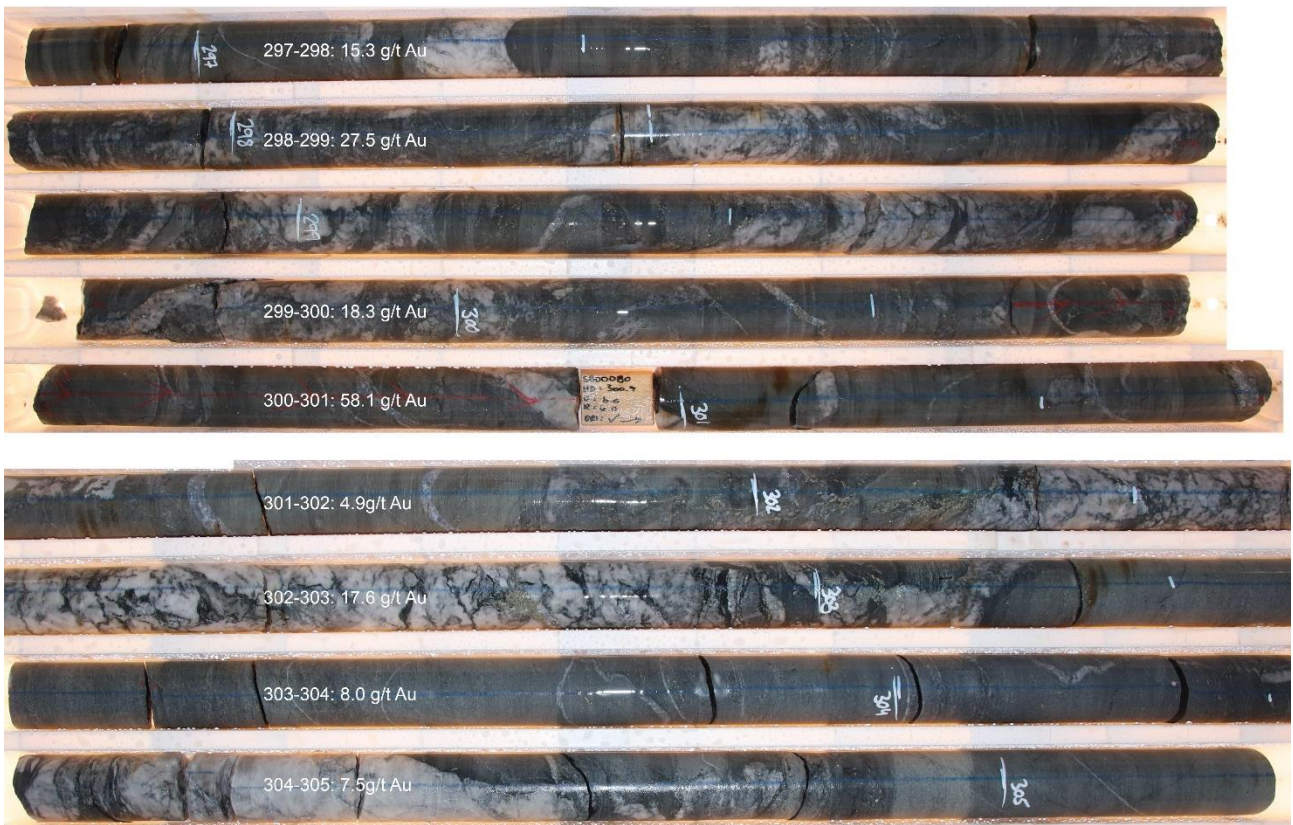
Figure 2: Photograph of mineralisation in hole SBDD080 with individual 1 metre gold assays shown in white.
