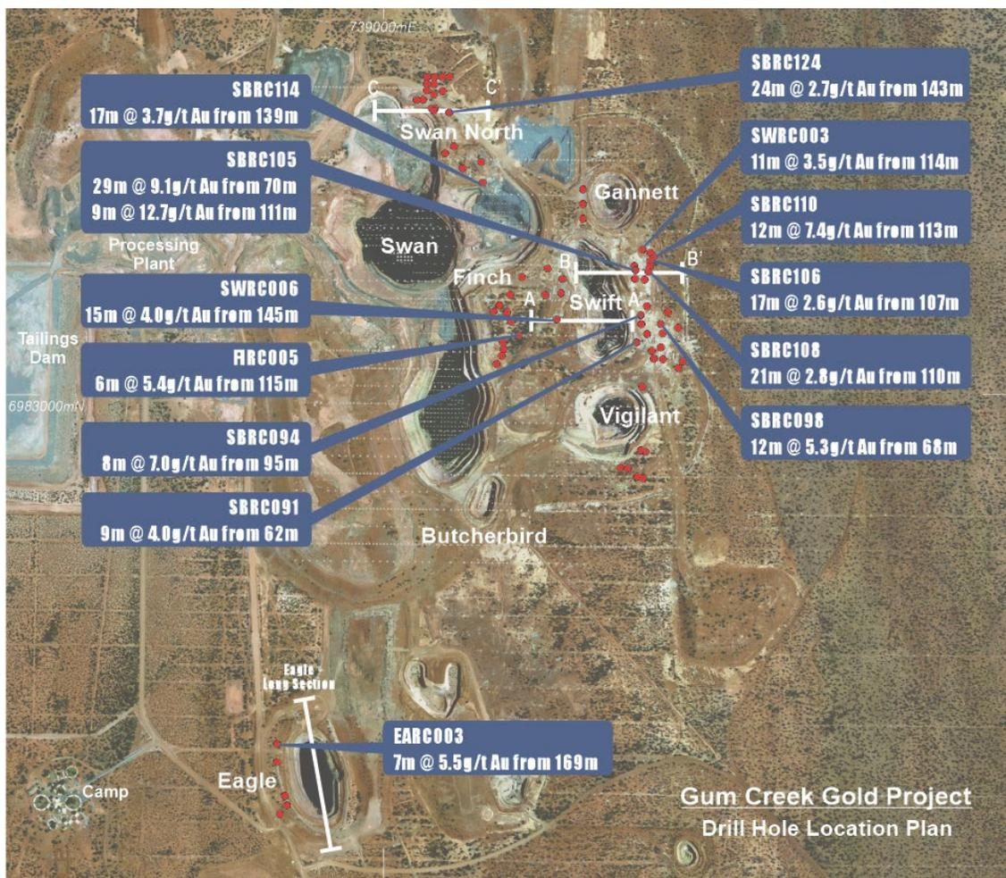
Figure 3: Eagle-Swift-Swan drill hole location plan with all FY2021 intercepts >30 GxM labelled.
