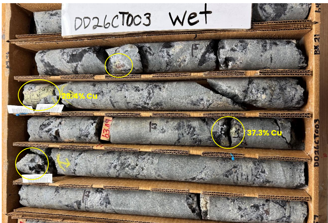
Figure 2: Chalcopyrite copper mineralisation and spot pXRF assays between 62.5–64.5m down hole DD26CT003
