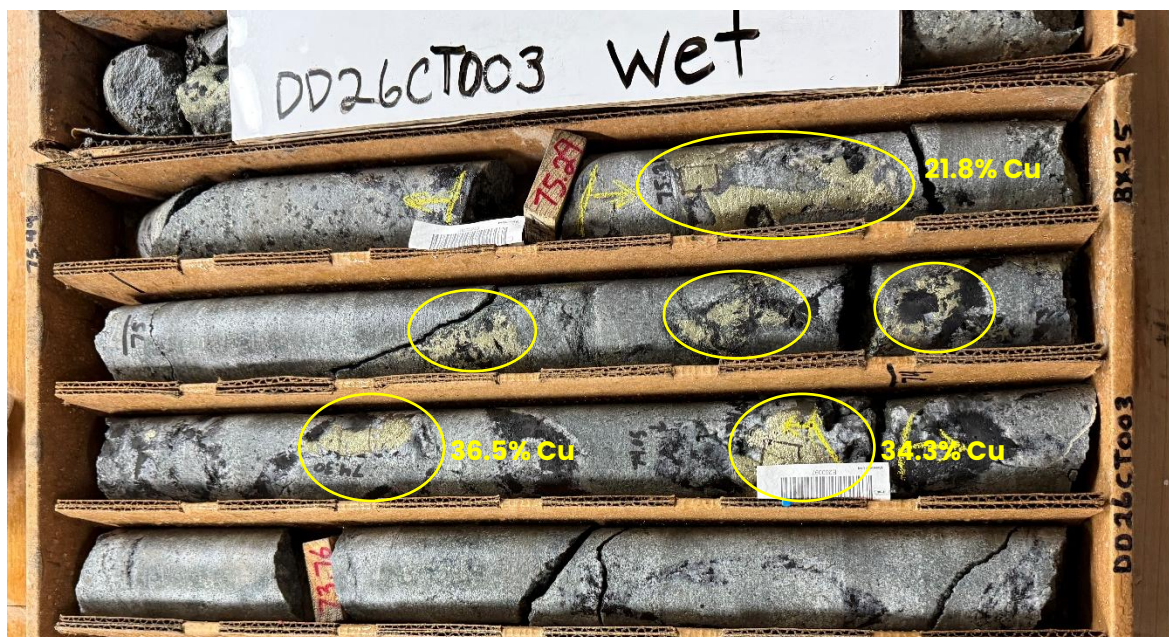
Figure 1: Visible chalcopyrite copper mineralisation between 74–76m down hole DD26CT003 with spot pXRF copper assays.
