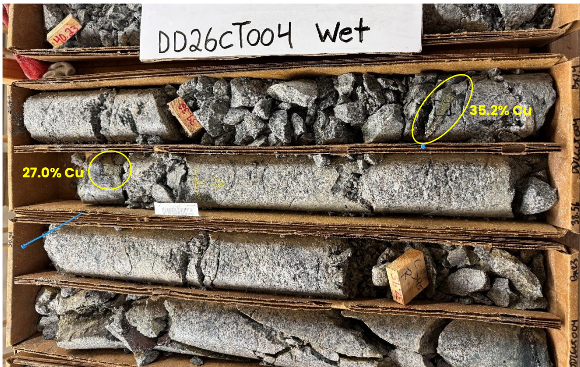
Figure 3: Chalcopyrite copper mineralisation and spot pXRF copper assays between 37.0–39.5m down hole DD26CT004
