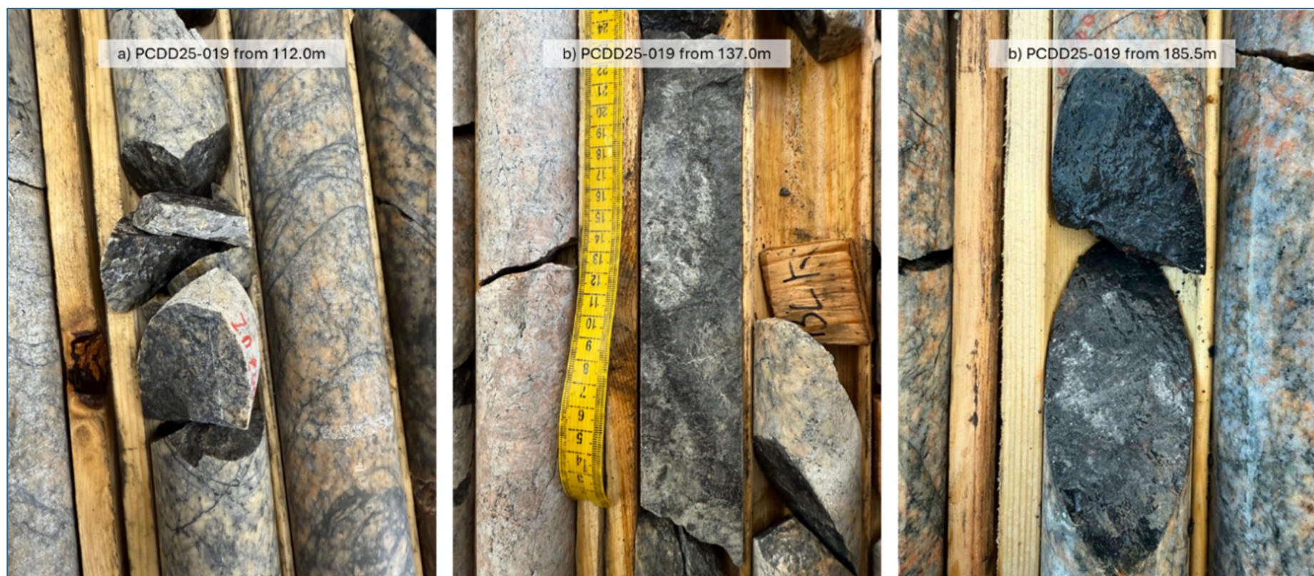
Figure 5: Drill core from PCDD25-019 (470813E, 5558967N, UTM Zone 21) demonstrating significant mineralisation of Zn, Cu and Mo in fractures.
