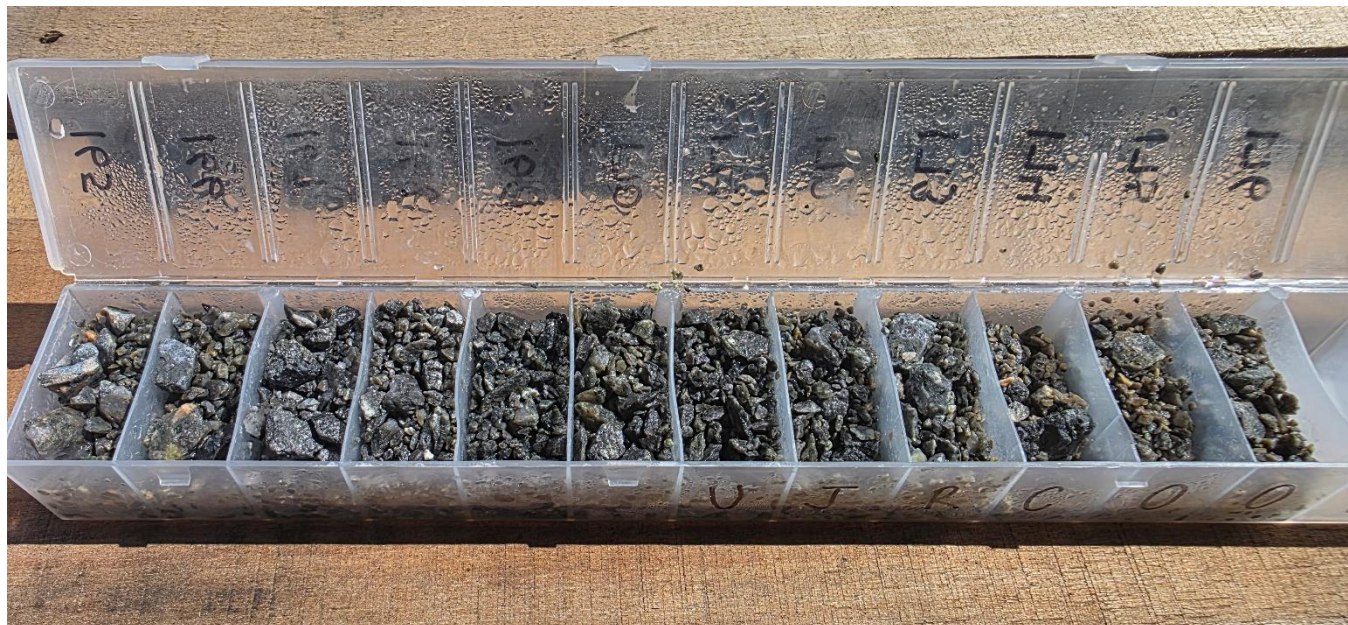
Figure 5 Union Jack Drill Hole UJRC002 Chip Tray (165m to 176m)
