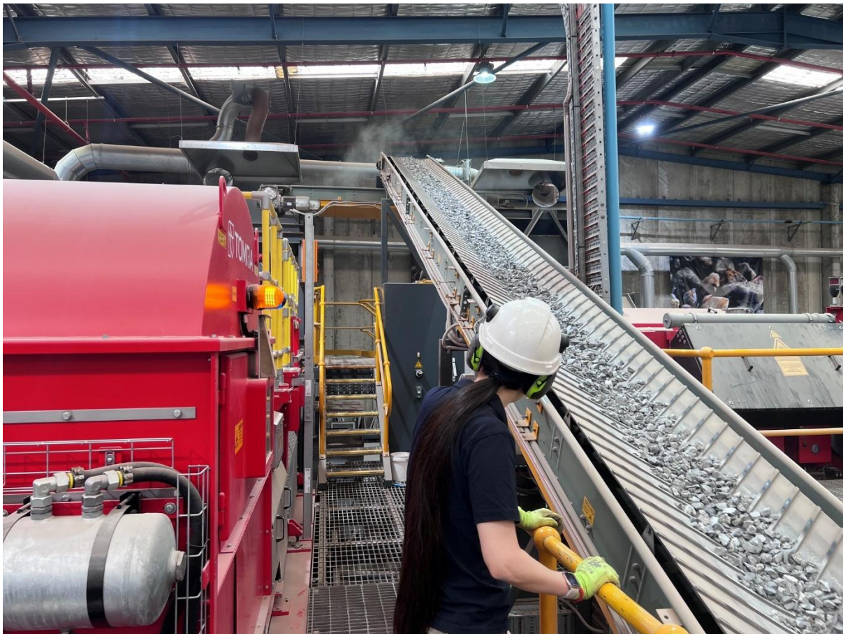
Figure 2 Orient bulk sample being fed into the TOMRA XRT ore sorter
