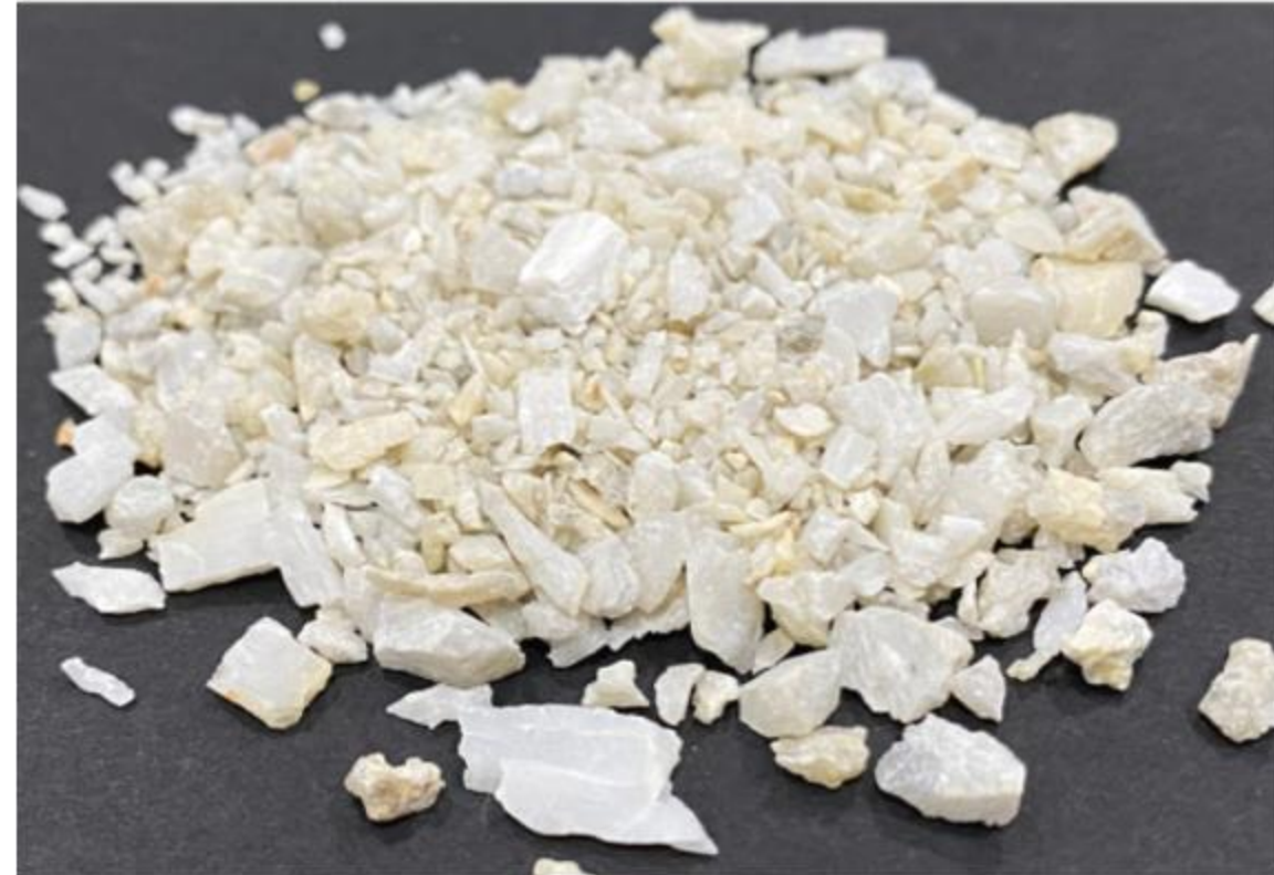
Photo of 6.1% \text{Li}_2\text{O} spodumene concentrate generated from mineralised materials sourced from drill hole BDD-24-022, Sample 2 at the Beecher Project 7
